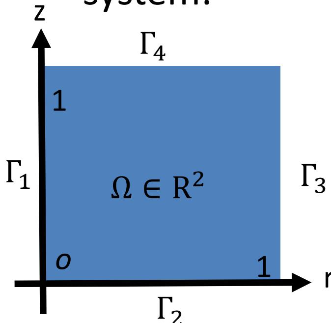
$$\frac{\partial^2 u}{\partial r^2} + \frac{1}{r} \frac{\partial u}{\partial r} + \frac{\partial^2 u}{\partial z^2} = 0 \text{ in } \Omega$$
