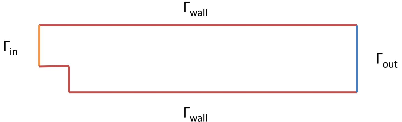
$$u = y(1 - y), v = 0, \frac{\partial q}{\partial n} = 0 \quad \text{on } \Gamma_{\text{in}}$$
