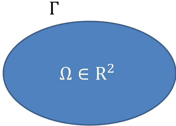
$$\begin{aligned}-\Delta u - f &= 0 \text{ in } \Omega \\ u &= 0 \text{ on } \Gamma\end{aligned}$$
